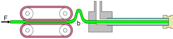
**Figure 6. Buckling of cable after drive belt**
