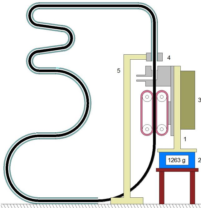
Figure 4. Schematics of calibration of pushing force
