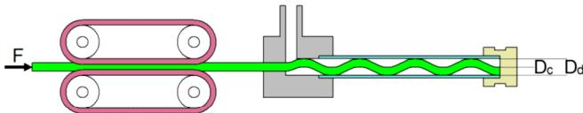
**Figure 7. Buckling of cable in duct**
