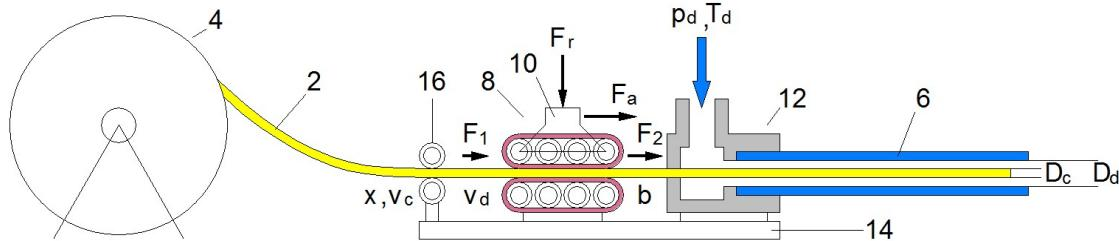
Figure 2. Functional drawing of “intelligent” jetting device
