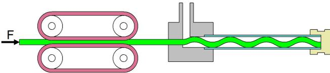
Figure 3. Crash test with buckling of cable in duct
