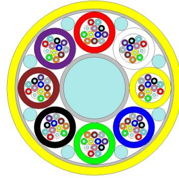
Figure 1. Example of microduct cable with 96 fibers
