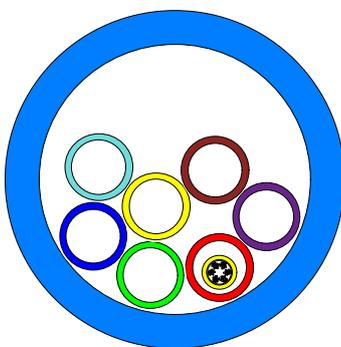
Fig. 14 Cross sectional view of duct with loose bundle of microducts
