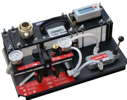
Fig. 9 First commercial cable blowing machine
