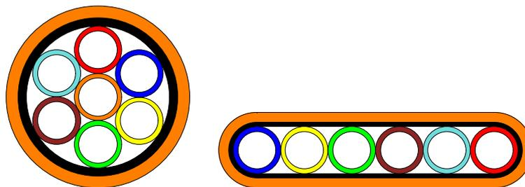
Fig. 17 Cross sectional view of examples of tight-bundled of microducts
