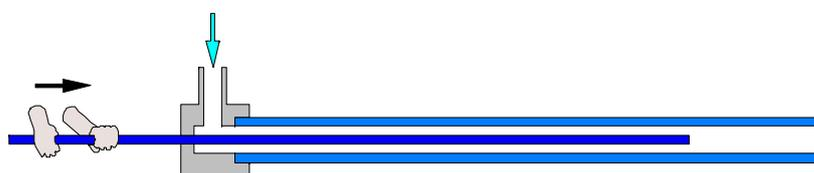
**Fig. 6 Manual test to evaluate blowing of real cables**
