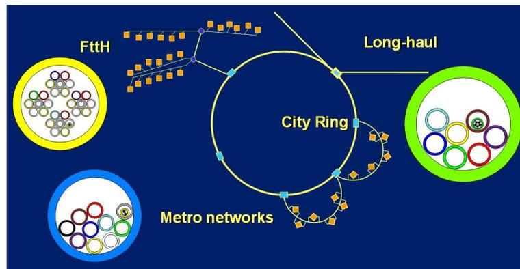
Fig. 16 Schematic view of access network, with redundant primary ring and redundant secondary half-rings for business customers.
