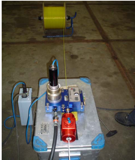
Figure 2: Blowing the preferrulized cable into a 4/3 mm microduct.
