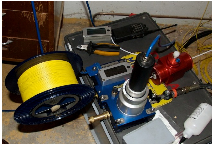
Figure 6: Blowing from a small spool.
