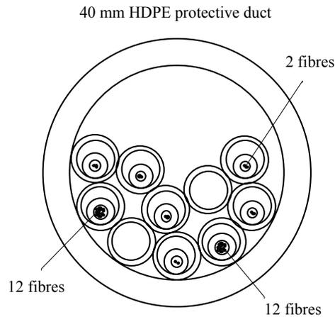
**Figure 7** Cross-sectional view of tubes and cables for network-structure of Figure 6.
