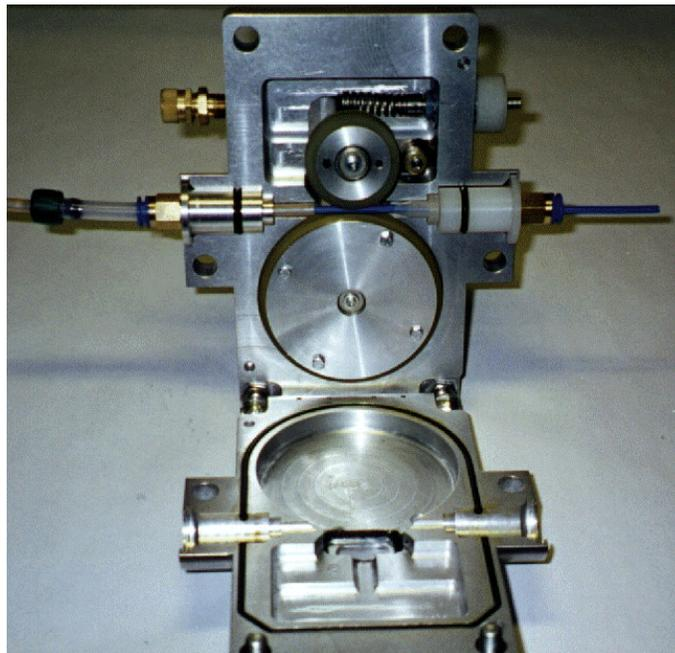
**Figure 4** Microjet<sup>®</sup>, installation unit for blowing cables into guide-tubes.
