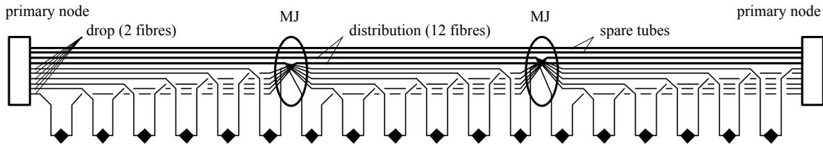
**Figure 6** Example of 18 double-routed connections through one 40 mm protective duct using joints (MJ's).
