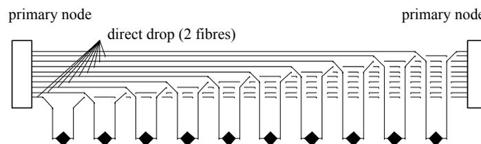
**Figure 5** Example of 10 double-routed connections through one 40 mm protective duct.
