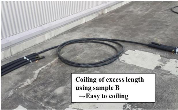
Figure 11. Coiled status of the 3456f slotted core cable
