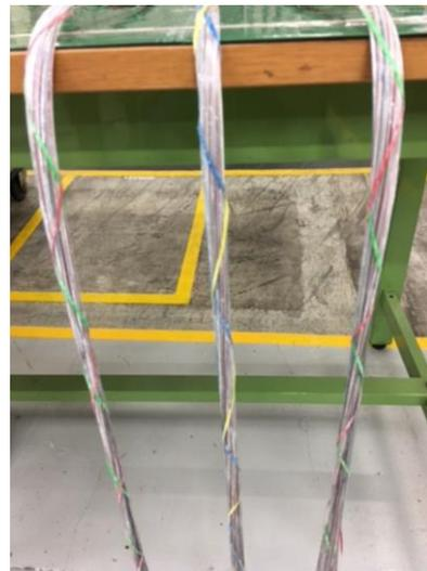
Figure 5. Picture of subunits bound by color tape in UHFC cable
