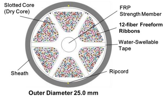
Figure 12. Cross-sections of UHFC cable samples for blowing tests
