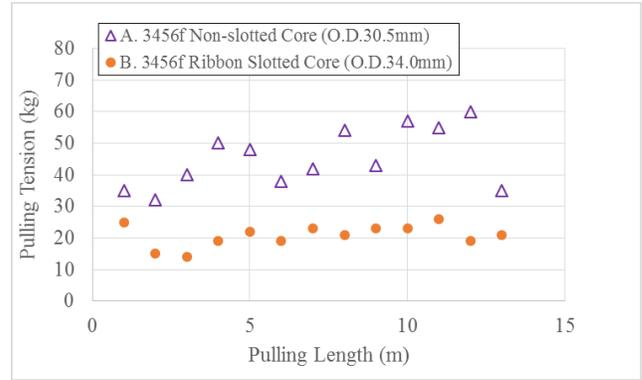
**Figure 9. Pulling test result of UHFC cables**
