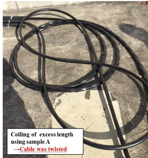
**Figure 10. Coiled status of the 3456f non-slot cable**
