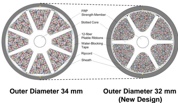
Figure 3. Cross-section of 3456-fiber count cable
