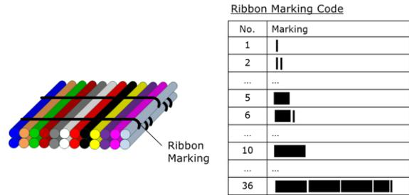
Figure 4. Schematic diagram of a ribbon identification pattern for UHFC cable
