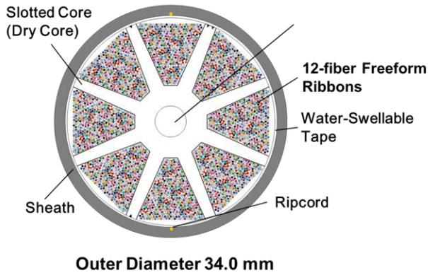
**Figure 7. Cross-sections of UHFC cable samples for installation tests**
