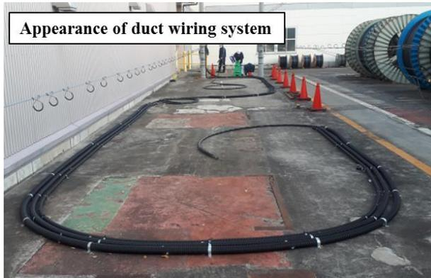
**Figure 8. Scheme of cable installation test**
