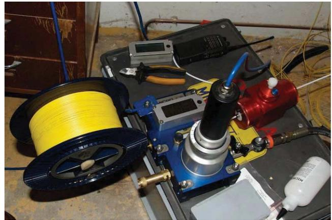
Figure 12. Blowing from a small spool
