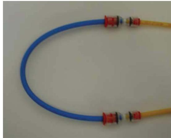
**Figure 16. Bend of 5/3.5 mm microduct placed in between 4/3 mm microduct sections**
