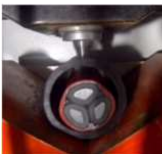
Fig. 6: Impact test on unarmoured cable in pipe
